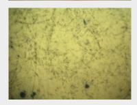
Cracks in case precoat is too brittle.
